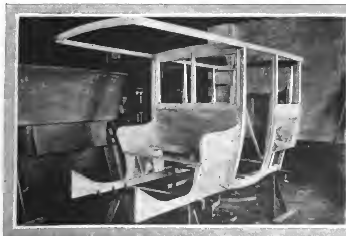
WOOD AND ALUMINUM BODY UNDER CONSTRUCTION.
